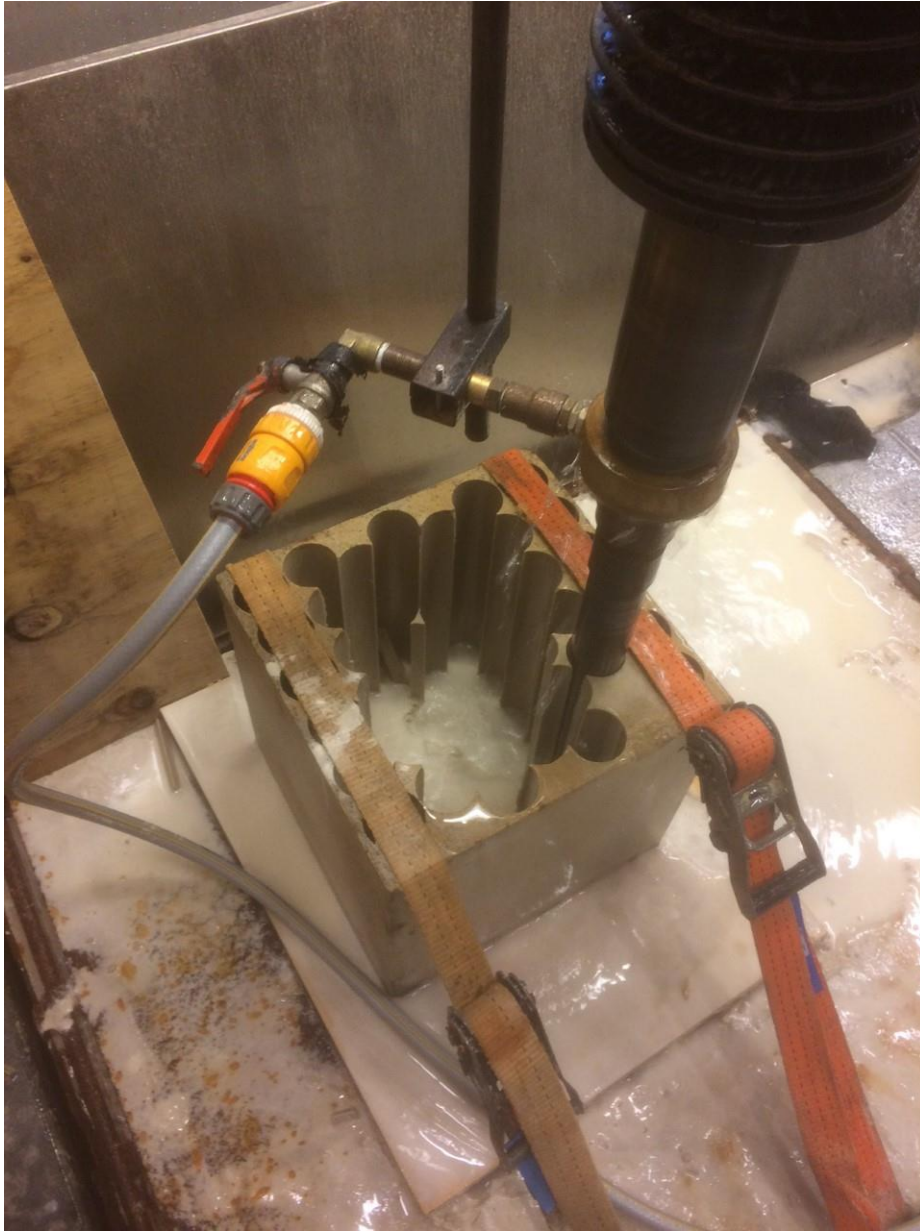
Figure 16 Cores being drilled out of a 40cmx40cmx30 cm block by Ronny Håland, UTC. (Photo: Ronny Håland).
