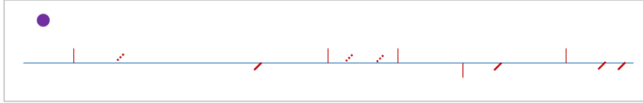
Figure 9 A simple model illustrating the dimensions of the polymer with grafting density 0.17% described by Hourdet et al. (1994). Scale ~1:50 000. The purple circle has the radius of the calculated random coil of the backbone. The blue line represents the contour length of the acrylic acid backbone and the red lines represent the contour length of the PEO-side chains. The thicknesses of the lines are not to scale.
